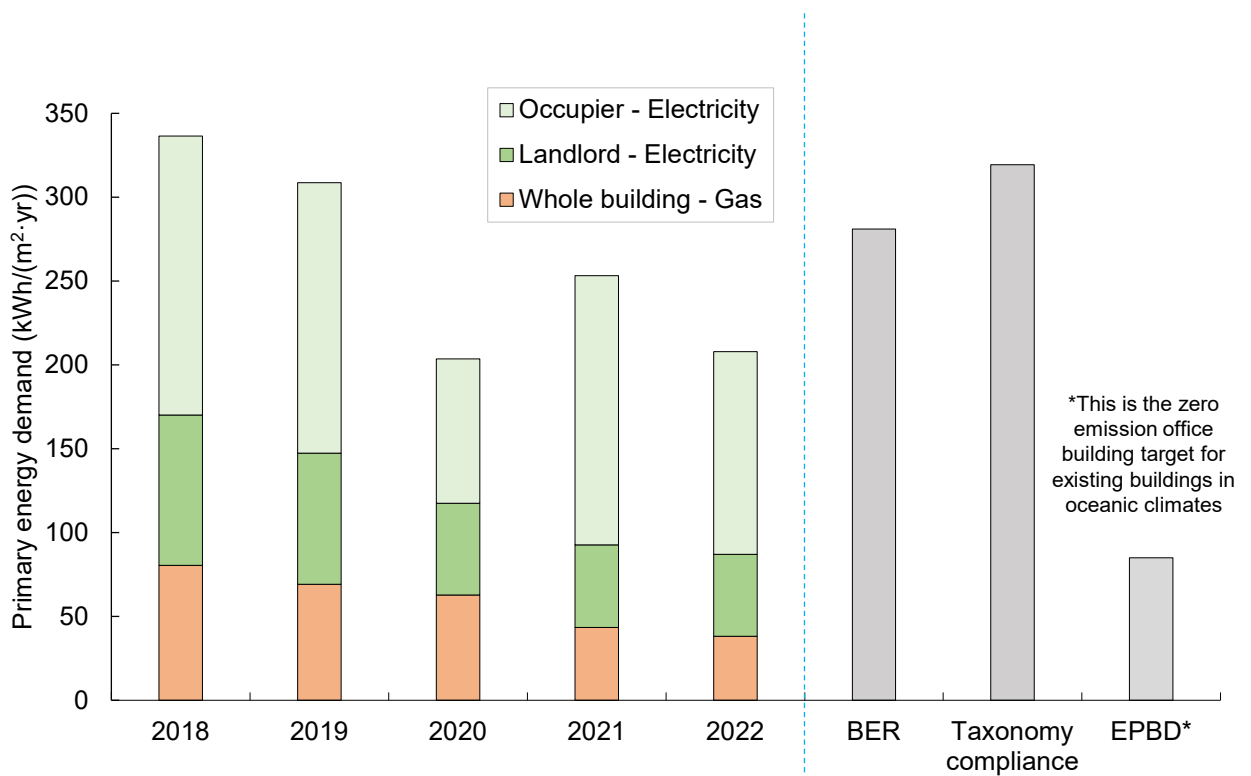
Figure 8. Primary energy demand for 1 Cumberland place between 2018 and 2022, compared with 1) its rated BER, 2) the requirement for EU taxonomy compliance as derived in Figure 7 and 3) the Zero Emission building target as per the latest EPBD.
